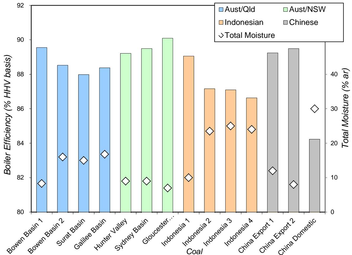
Figure 2: Calculated boiler efficiency for selected coals<sup>2</sup>
